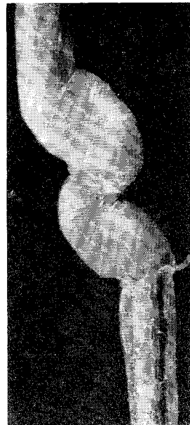
Fig. 7 Kinking of zinc by high-amplitude sound waves (amplitudes greater than 50 w/cm 2 )
